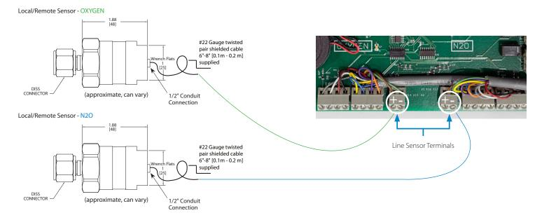
· Identify the appropriate gas sensor wire and connect it into the appropriate terminal, taking attention to the polarity
